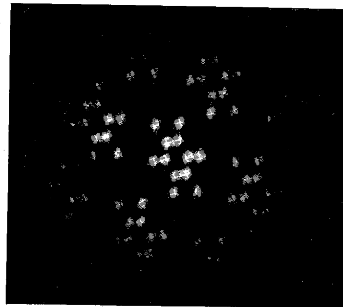
Fig. 6. Optical synthesis of molecules of hexamethyl benzene.
