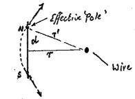
less than the physical length). For  $d\sim0.3$  cm., r=1cm., the "correction" is quite appreciable ( $\sim20\%$ ), and easily seen in careful measurements.
