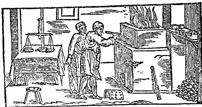
An assaying laboratory, showing balances, muffle furnace for cupeling, ingot mould, etc.
